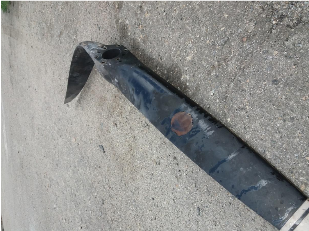
Picture 3 (damage to the propeller)
