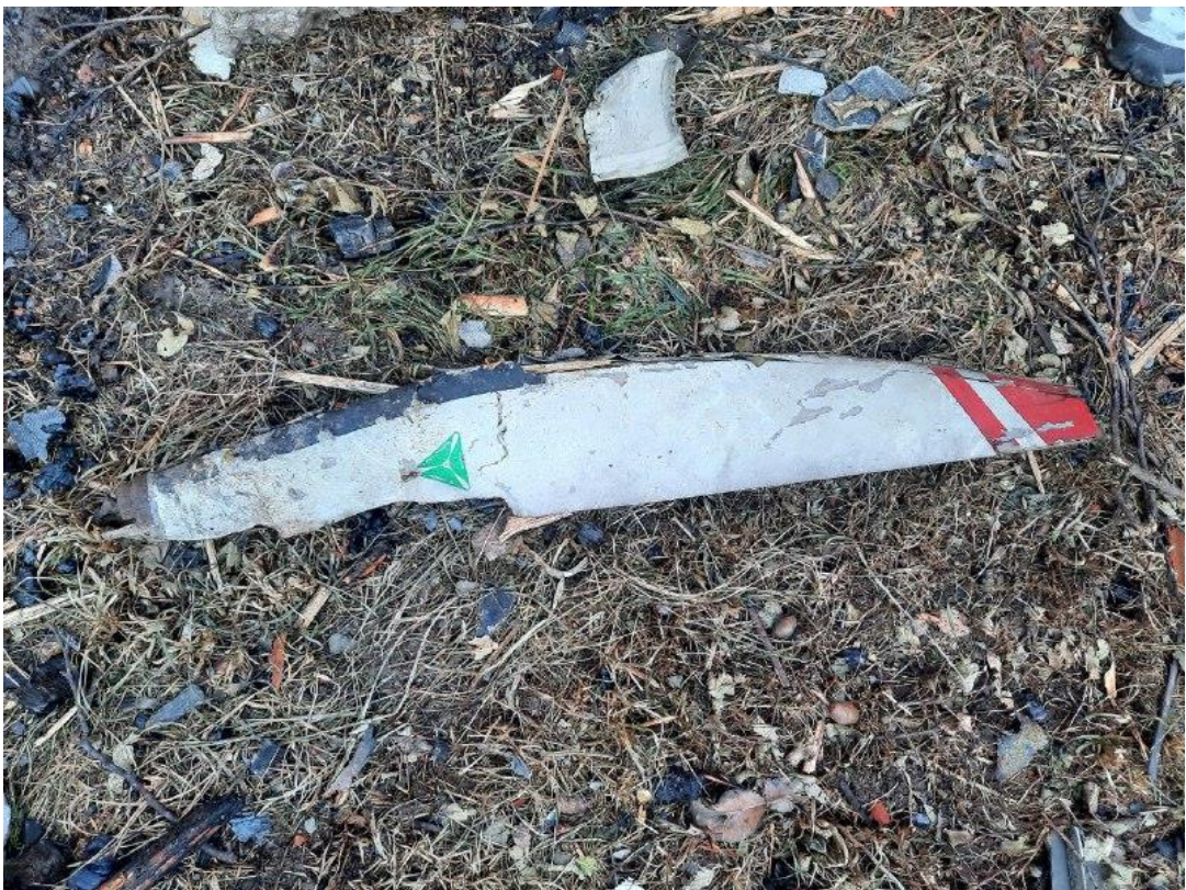
(Picture 1 – fracture near the propeller sleeve)
