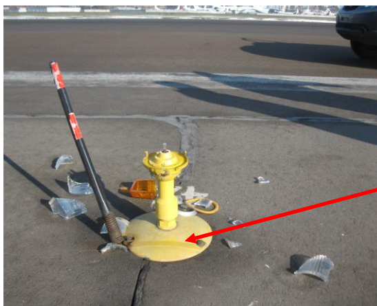
Fig. 4. Destroyed runway light No. 42.
